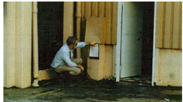
Photo 4: Photo record of April 1988 flood mark approximately 0.4m-0.5m above ground level (Source: Ref. 7).
